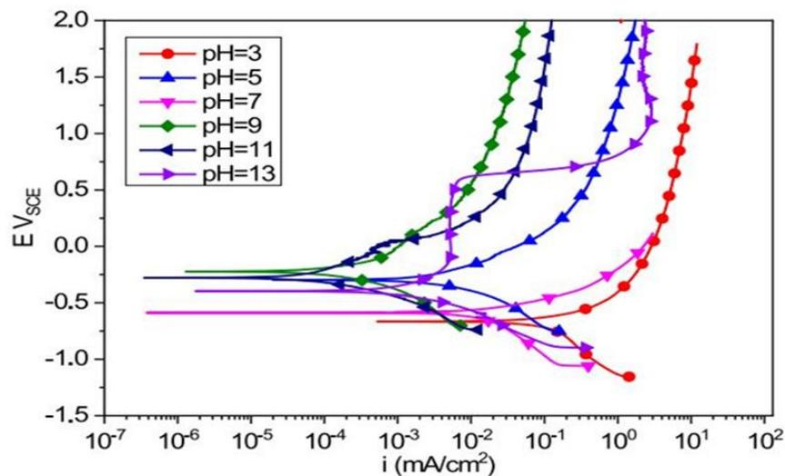
**Figure 7: Potentiodynamic polarisation curves of the MS specimens immersed at different pH ranging from pH=3 to pH=13 [3]**
