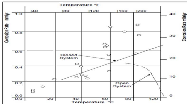
**Figure 2: Comparison of Actual Plant CUI Corrosion Rates Measurements with Laboratory Corrosion Data Obtained in Open and Closed Systems[4][5]**
