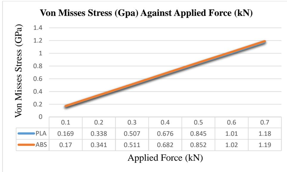
Figure 5: Graph Von Mises Stress against Applied Force for ABS and PLA Filament
