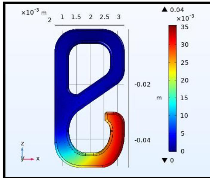
**Figure 7: Carabiner Displacement Using ABS Filament**
