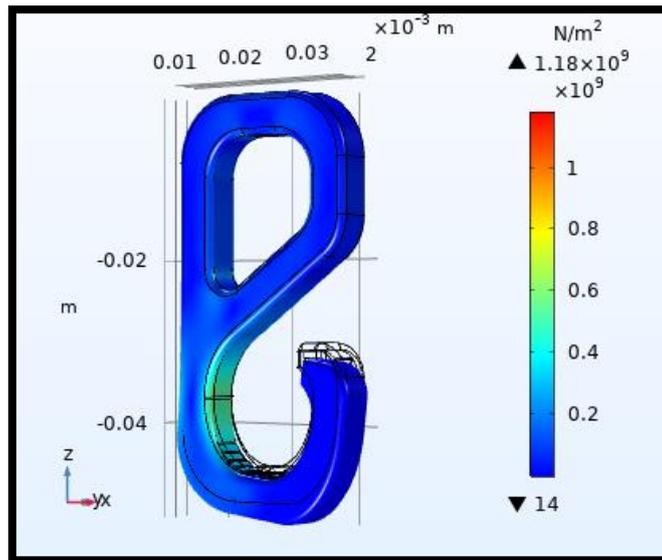
**Figure 3: Von Mises Stress for PLA Filament**
