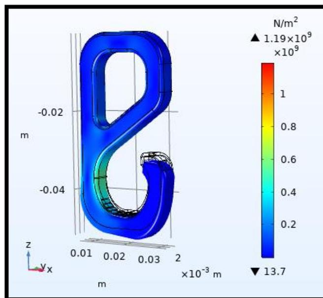
**Figure 4: Von Mises Stress for ABS Filament**
