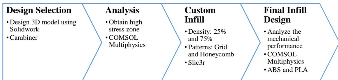
**Figure 1: Process from Design Selection until Final Infill Design**
