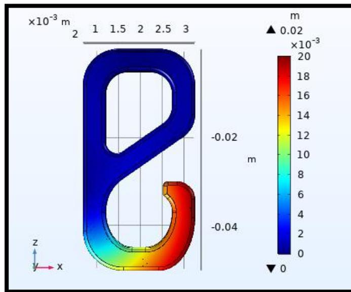
Figure 6: Carabiner Displacement Using PLA Filament
