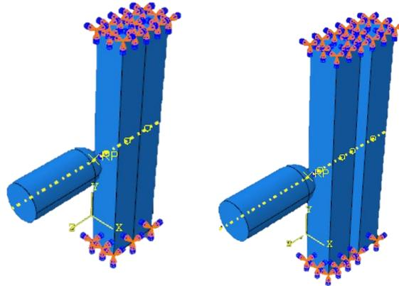
**Figure 5: Boundary condition set for the non-spaced cockleshell target plate**
