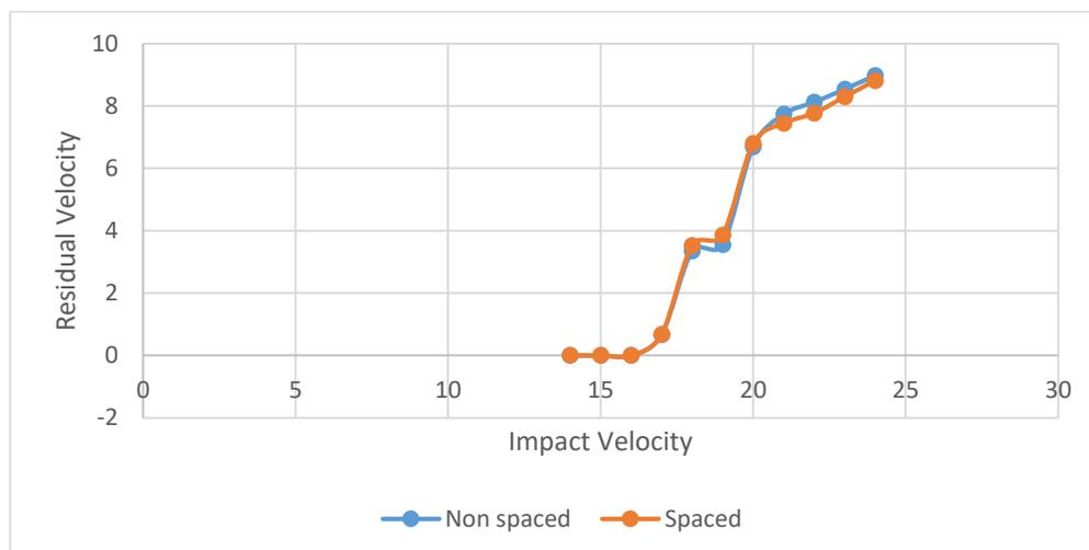
**Figure 8: Residual velocity vs Impact velocity of bullet after hitting both non-spaced and spaced plate**
