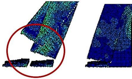
**Figure 14: Major fracture of cockleshell plate's endpoint**
