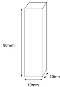
**Figure 1: 3D dimension of cockleshell target plate**
