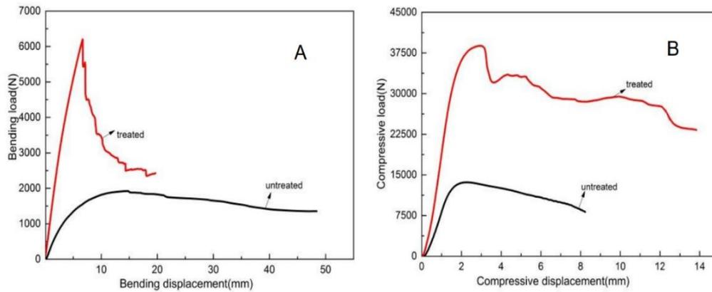
**Figure 3: Untreated and treated rattan mechanical load displacement: Bending load displacement (A) and compression load displacement (B)[11]**
