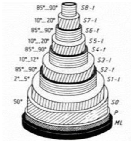
**Figure 1: Bamboo fiber multilayer structure model[2]**
