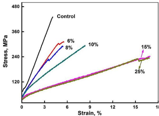
**Figure 2: Typical tensile stress–strain curves on individual bamboo fibers treated with varied concentrations of NaOH solutions[8]**
