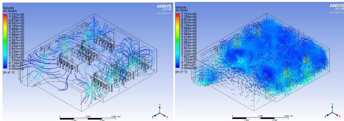
**Figure 5: The air velocity in analysis of air stream and air vector**
