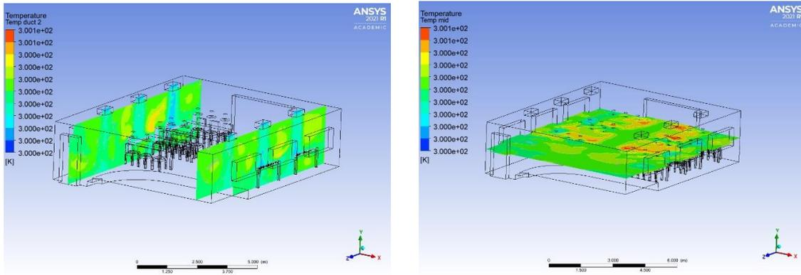
**Figure 3: The temperature distribution under the inlet and middle plane**
