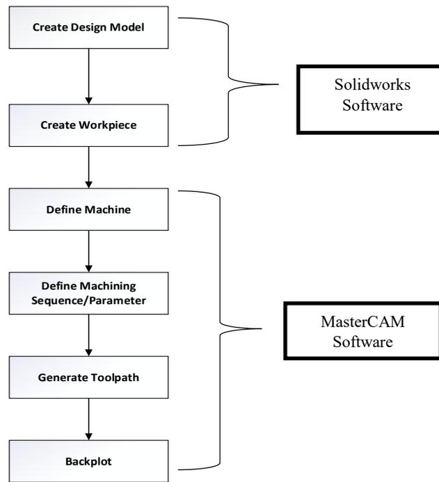
**Figure 3: Overall process using MasterCAM software**
