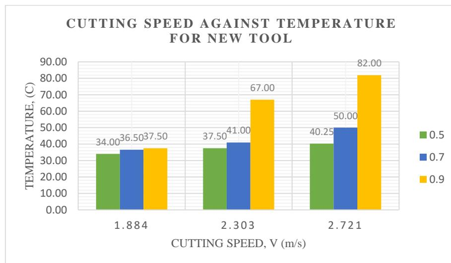
**Figure 4: Graph of Cutting Speed against Temperature for New Tool**
