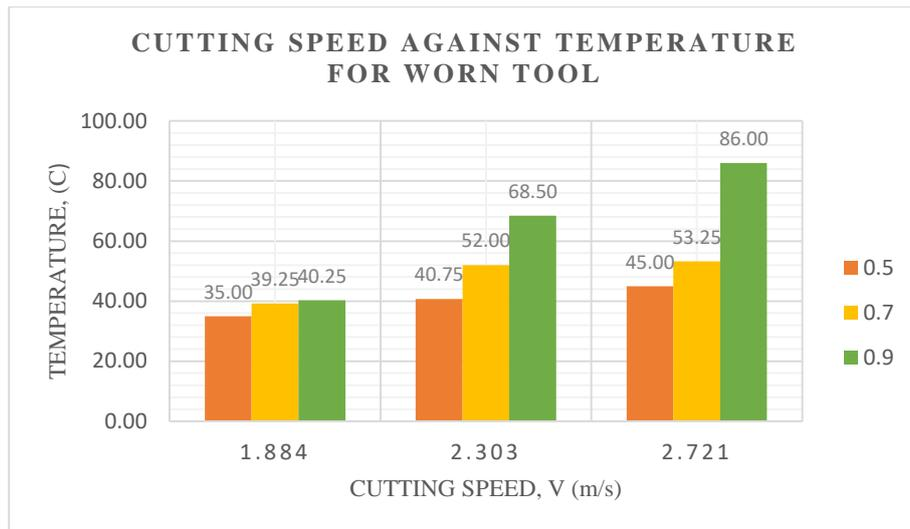
**Figure 5: Graph of Cutting Speed against Temperature for Worn Tool**
