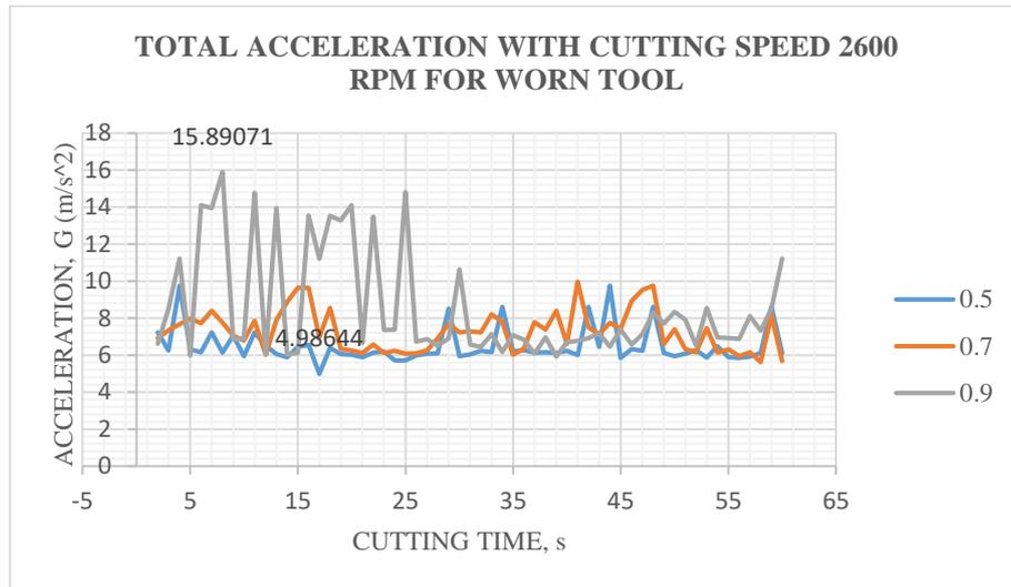
**Figure 7: Total Acceleration of Cutting Speed 2600rpm for Worn Tool**
