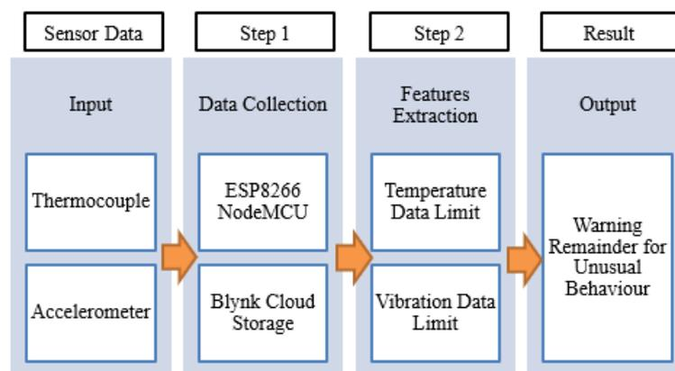
**Figure 2: Overview of the System Architecture**
