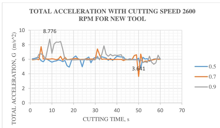
**Figure 6: Total Acceleration for Cutting Speed 2600rpm for New Tool**
