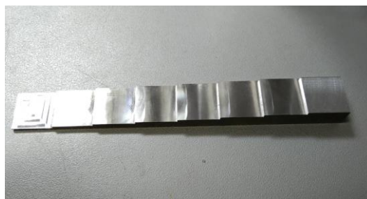
Figure 2: Custom 8 Step wedge block 304 stainless steel
