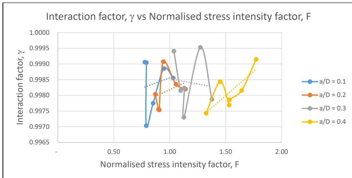
**Figure 7: Graph of interaction factor,  $\gamma$  against normalised stress intensity factor, F**
