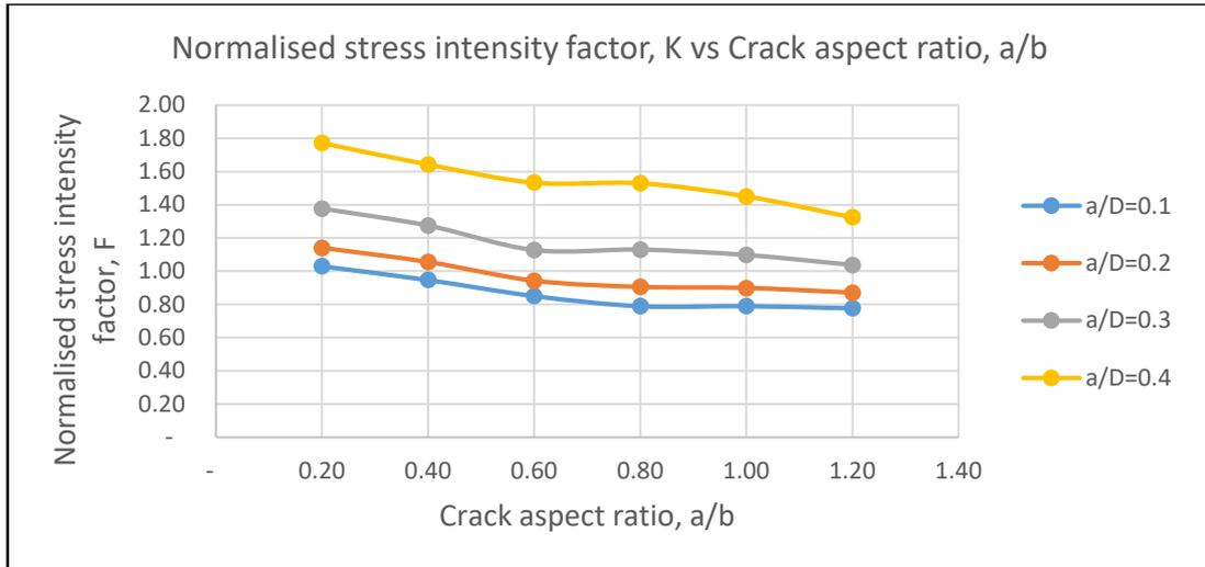
**Figure 5: Graph of normalised stress intensity factor, F against crack aspect ratio, a/b**
