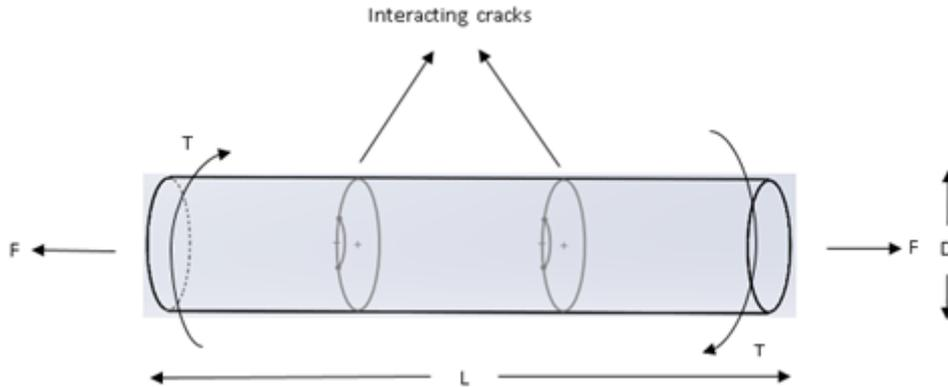
**Figure 1: Diagram of two interacting cracks on a cylindrical rod**
