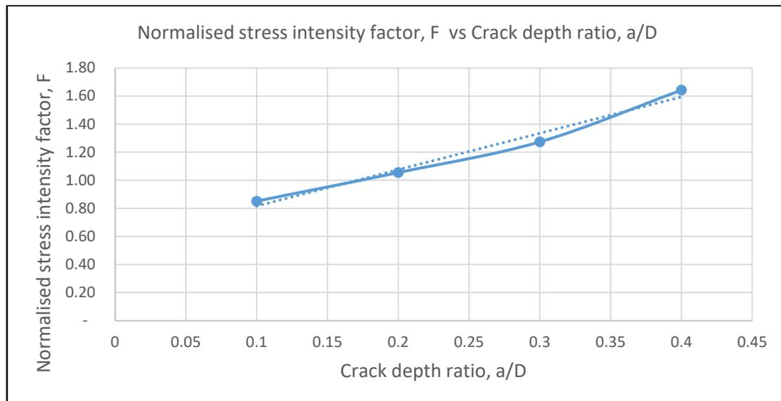
**Figure 4: Graph of normalized stress intensity factor against crack depth ratio**
