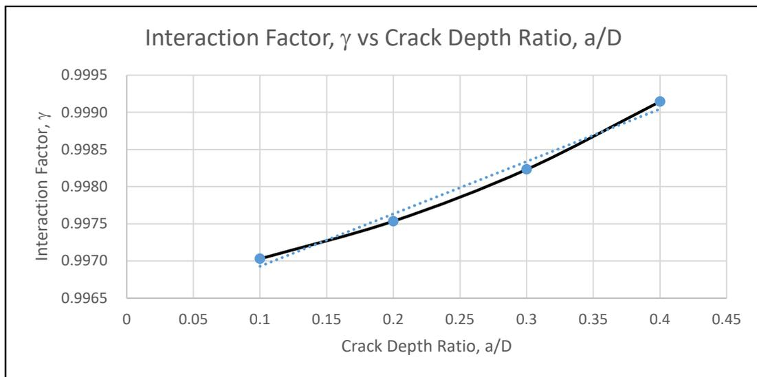
**Figure 6: Graph of interaction factor, γ against crack depth ratio, a / D**
