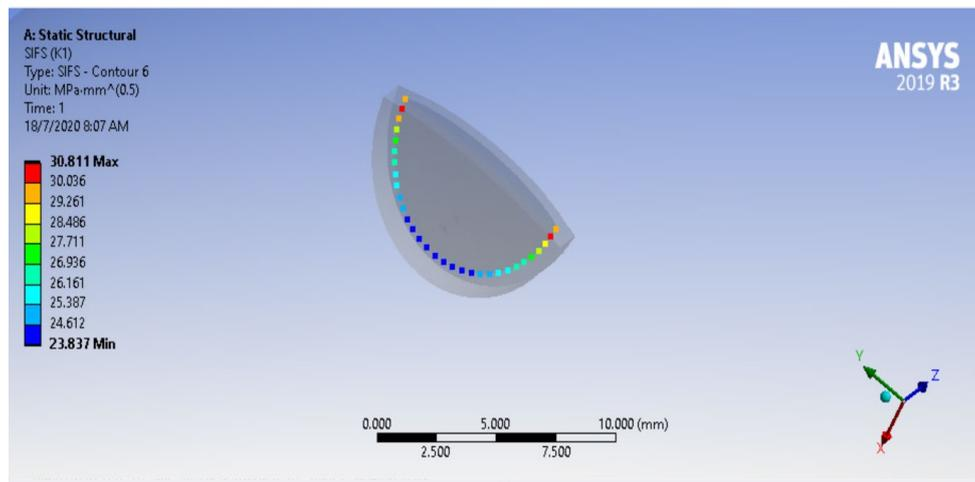
**Figure 3: Example of simulation results ( $a/D = 0.1$ ;  $a/b = 1.2$ )**
