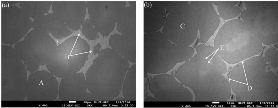
**Figure 3: SEM micrographs for ZRE1 base alloy and ZRE1 alloy treated with 1.75 wt.% Er [6]**
