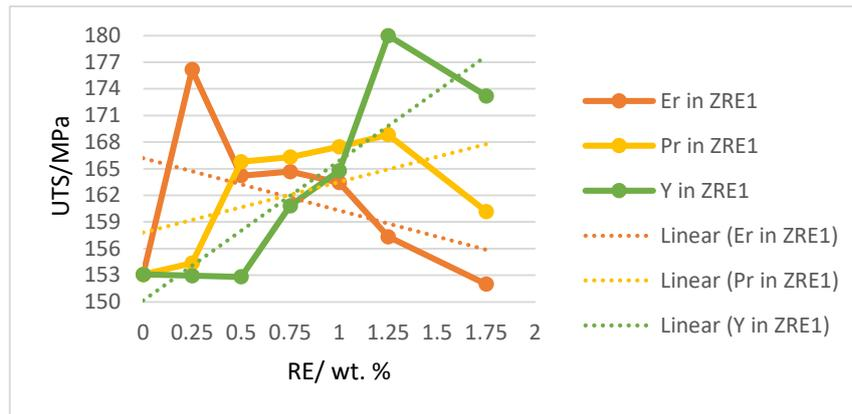
**Figure 4: Effect of RE additions on UTS values for ZRE1 alloys**
