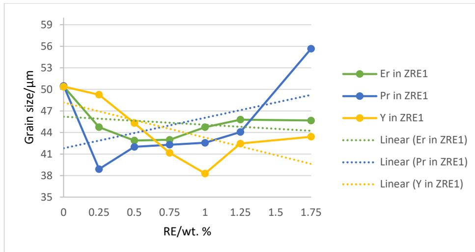
**Figure 1: Effect of the additions of RE on the grain sizes of ZRE1 magnesium alloy**
