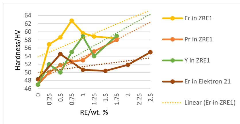
**Figure 5: Effect of RE additions on the hardness values of magnesium alloys**
