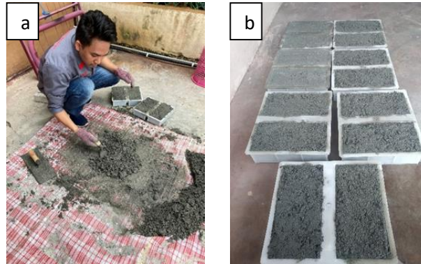
Figure 3: (a) The mixture poured and compacted into the mould. (b) All specimen already put into mould.
