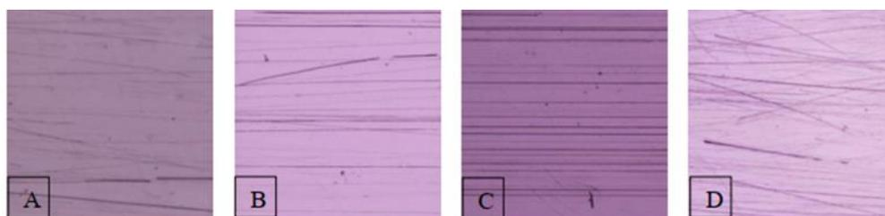
**Figure 10: Cockle shell waste brushing cycle scratch pattern (A= 0.5cycle, B= 1cycle, C=10cycles, D=20cycles)**
