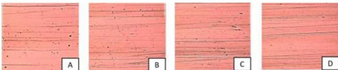
**Figure 5: Oyster shell waste brushing load scratch pattern (A= 0N, B=1.0N, C=1.5N, D=2.0N)**
