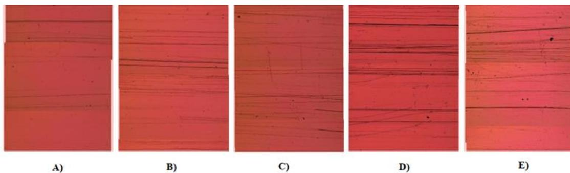
**Figure 3: Mussel shell waste brushing load scratch pattern (A= 0N, B= 0.5N, C=1.0N, D=1.5N, E=2.0N)**
