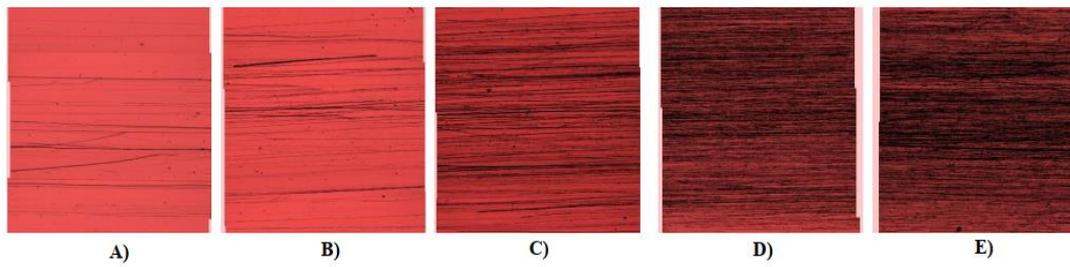
**Figure 7: Mussel shell waste brushing cycle scratch pattern (A= 0.5cycle, B= 1cycle, C=5cycles, D=25cycles, E=50cycles)**
