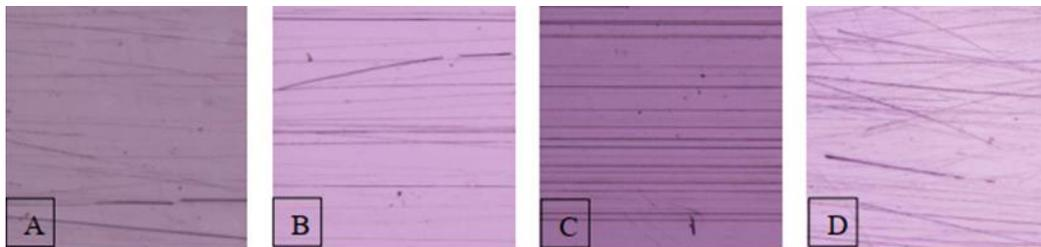
**Figure 6: Cockle shell waste brushing load scratch pattern (A= 0N, B=1.0N, C=1.5N, D=2.0N)**
