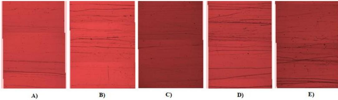
**Figure 4: Clam shell waste brushing load scratch pattern (A= 0N, B= 0.5N, C=1.0N, D=1.5N, E=2.0N)**
