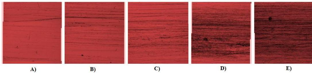
**Figure 8: Clam shell waste brushing cycle scratch pattern (A= 0.5cycle, B= 1cycle, C=5cycles, D=25cycles, E=50cycles)**
