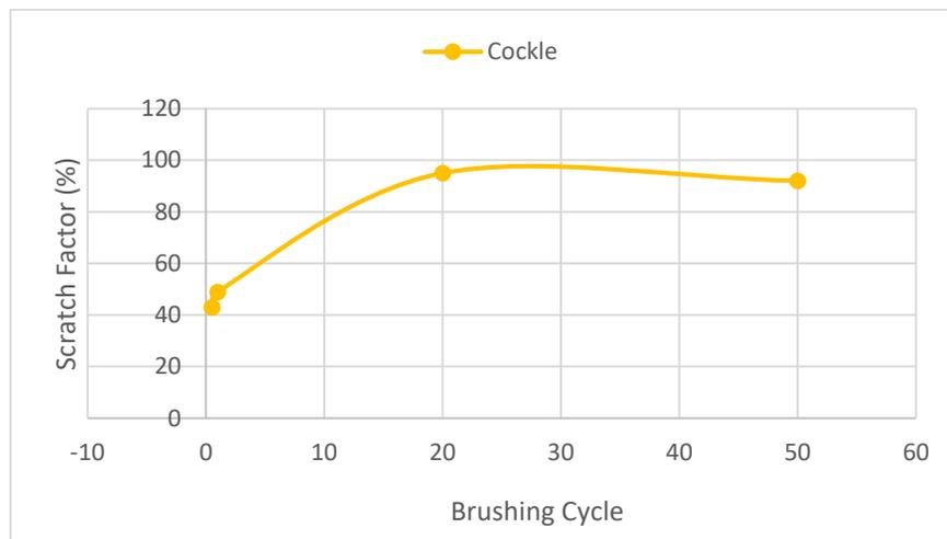
**Figure 2: Scattered graph of cockle scratch factor**
