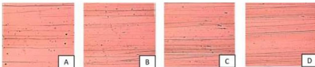
**Figure 9: Oyster shell waste brushing cycle scratch pattern (A= 0.5cycle, B= 1cycle, C=10cycles, D=20cycles)**
