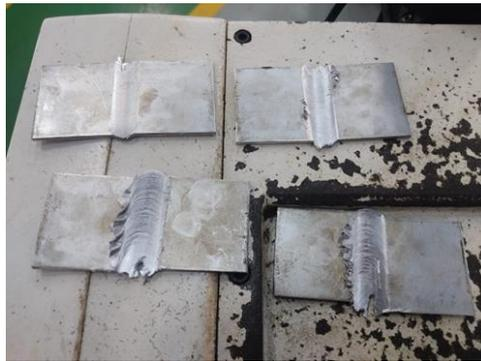
**Figure 3.2: Joint plate by friction stir welding with different parameters**
