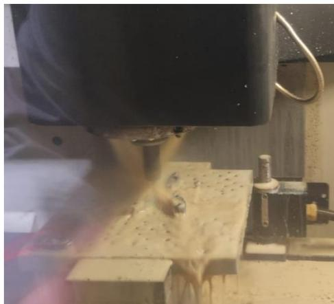
**Figure 3.5: Dog bone production in progress by using CNC Vertical Milling Machine**
