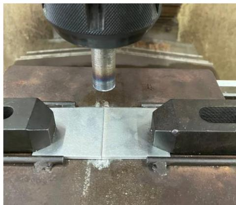
**Figure 3.1: Base material is clamped before welding process**
