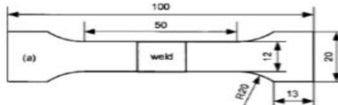
**Figure 3.4: Dog bone design from ASTM D3039 requirement**
