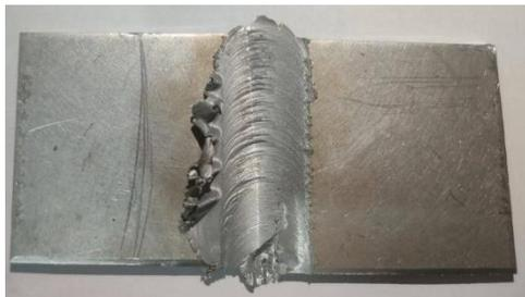
**Figure 3.3: Welding defects in friction stir welding**
