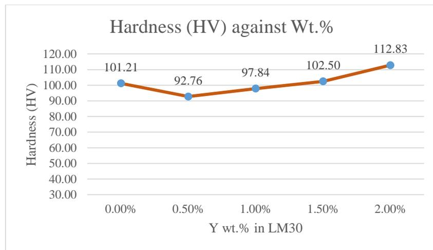
**Figure 5: The effect of Y addition on the hardness values of LM30 aluminium alloy**
