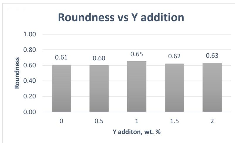
Figure 4: Graph of Roundness versus Y addition, wt. %
