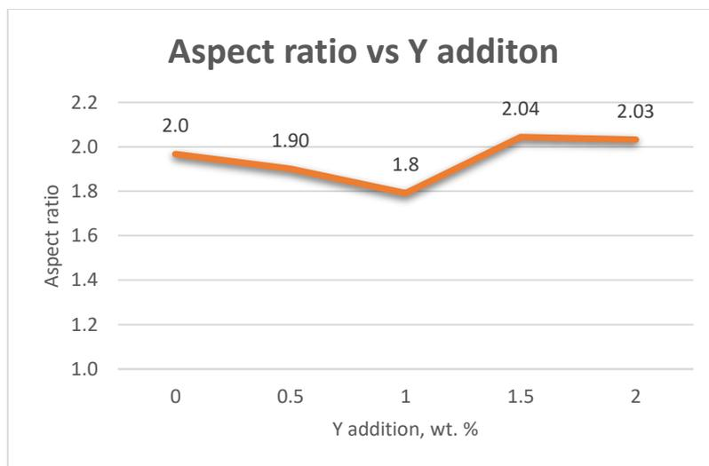
Figure 3: Graph of Aspect Ratio versus Y addition, wt. %
