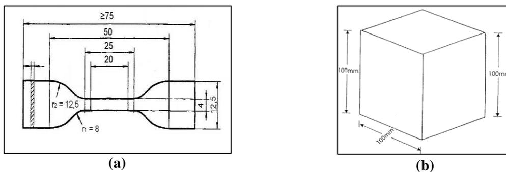
**Figure 1: Drawing on Dumbbell and Cube 0% infill**
