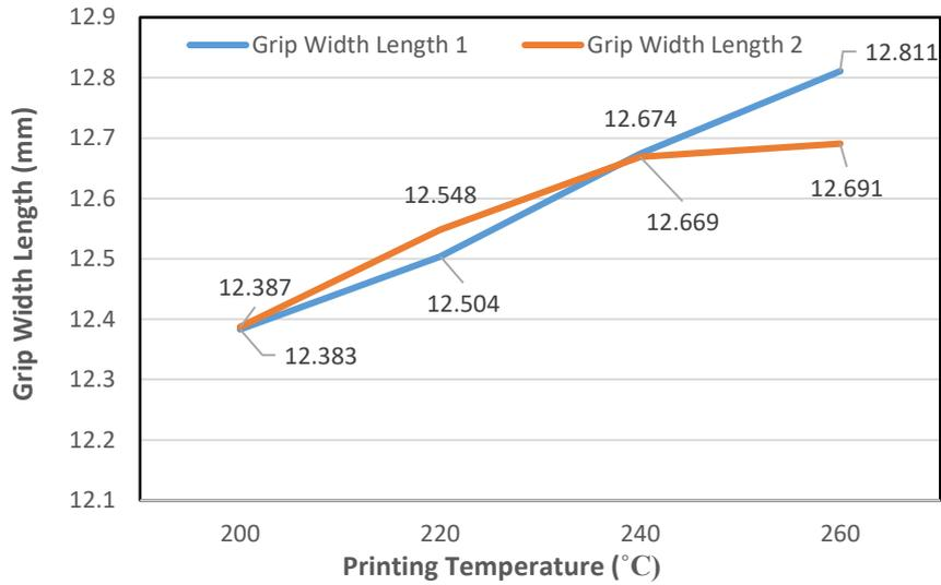
**Figure 3: Expansion Grip Width Length of Dumbbell**
