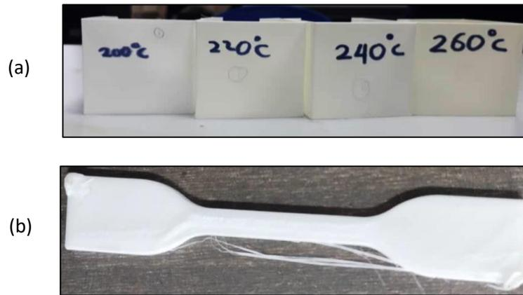
**Figure 1: The appearance of (a) a printed sample of cube 0% infill and (b) a dumbbell ISO527**
