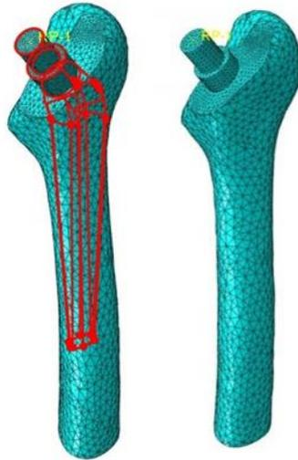
**Figure 3: Completed mesh on the initial design**
