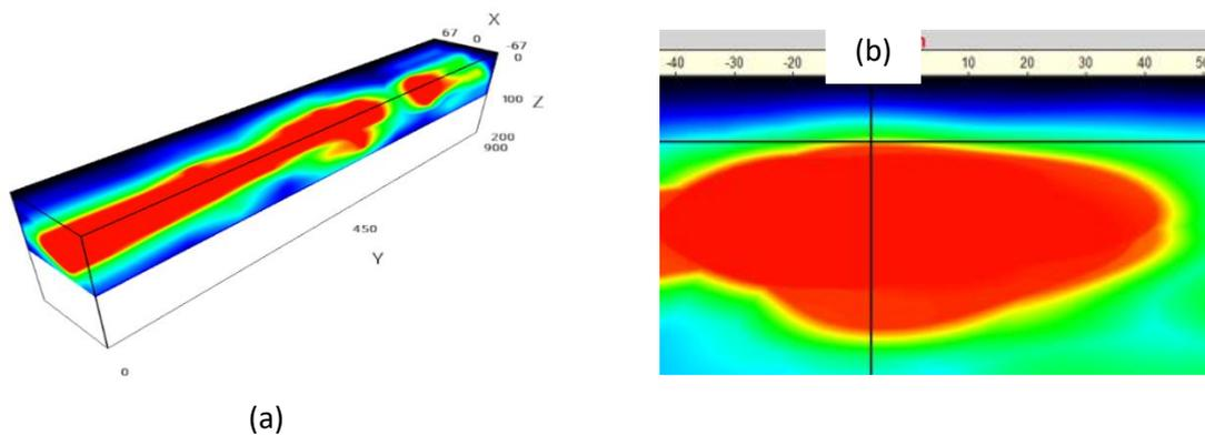
**Figure 9: (a) Results of case study 2(condition 2) (b)B-scan that show the steel bar slightly on the left of the phase array probe**
