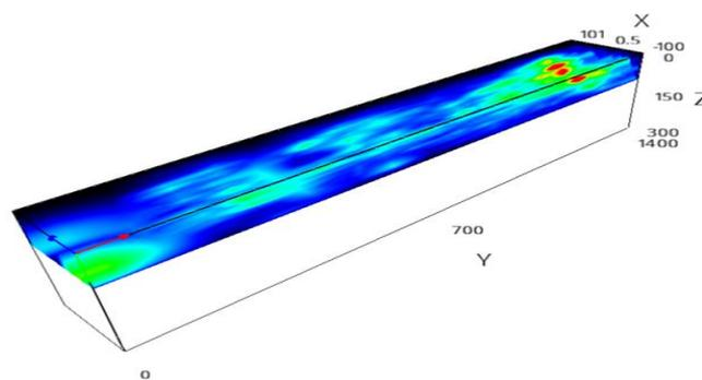
**Figure 11: The result of concrete structure expected to be no having a steel bar**
