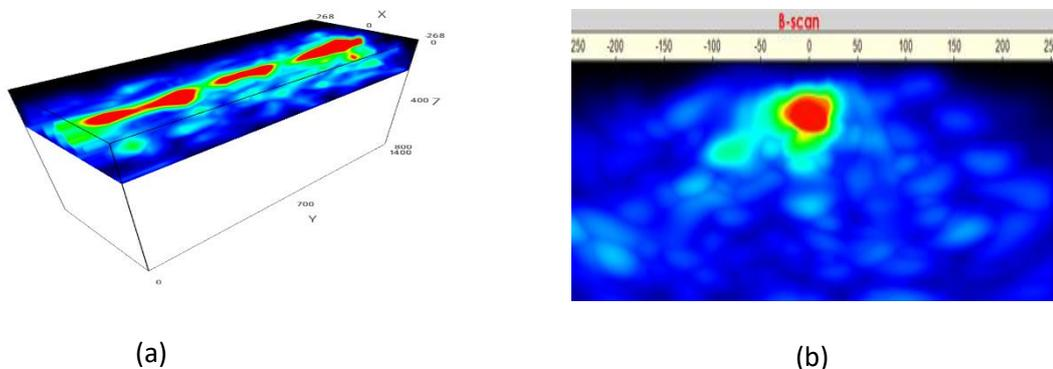
**Figure 7: (a) Results of case study 2 condition 1 (b)B-scan that show the steel bar in the mid of the phase array probe**
