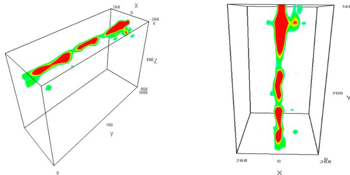
**Figure 8: The isometric and top view of the steel bar in the concrete structure.**
