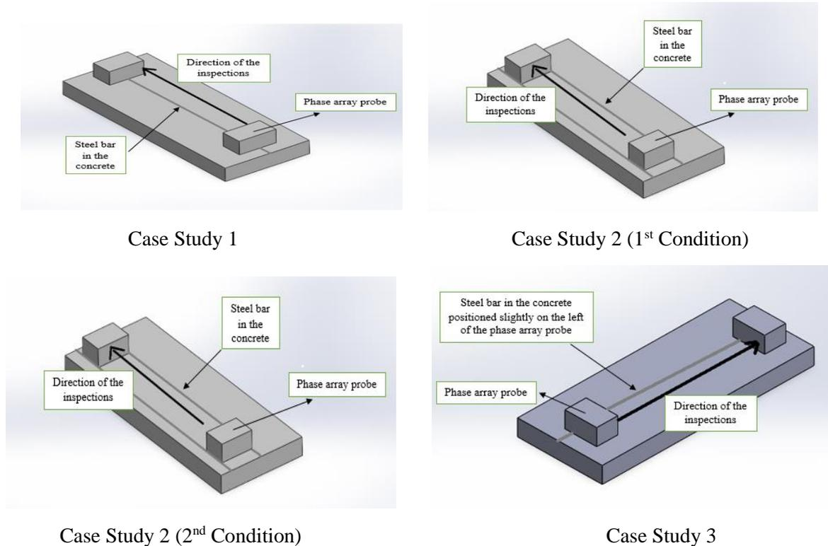
**Figure 2: Different case studies representing different arrangement of measurement**
