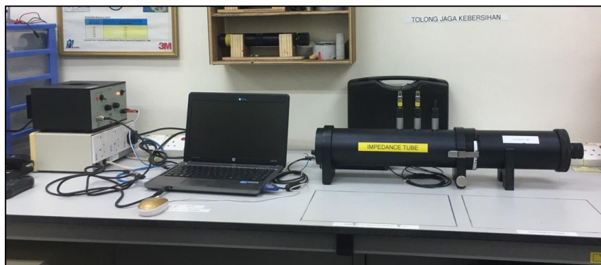
Figure 2: Experimental setup using impedance tube method
