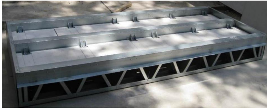
Figure 5: The assembled CFS trusses
