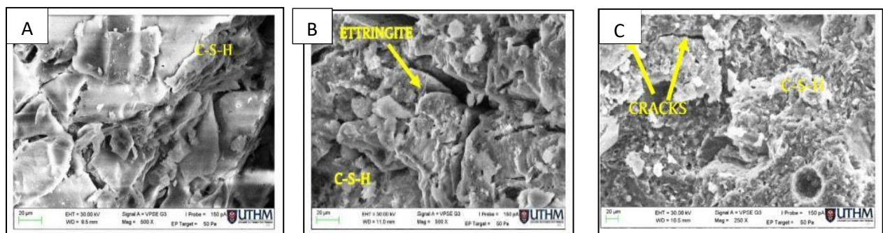
Figure 3: SEM image of concrete containing CBA under a) water condition b) 5% \text{Na}_2\text{SO}_4 solution c) 5% \text{NaCl} solution [35]
