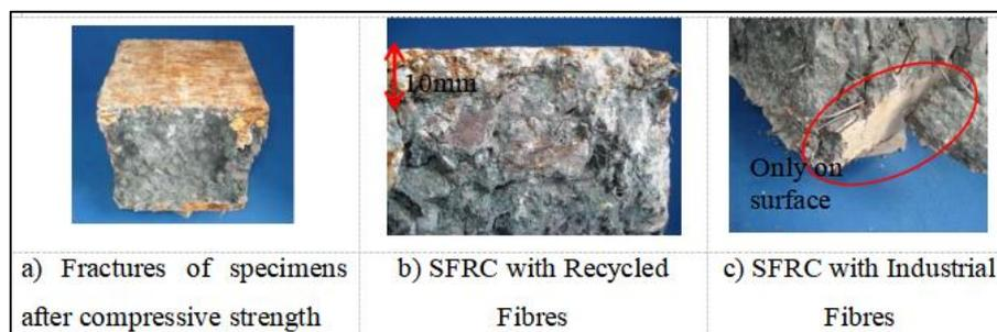
**Figure 5: Internal analysis of specimens after 5 months of accelerated corrosion test [11]**
