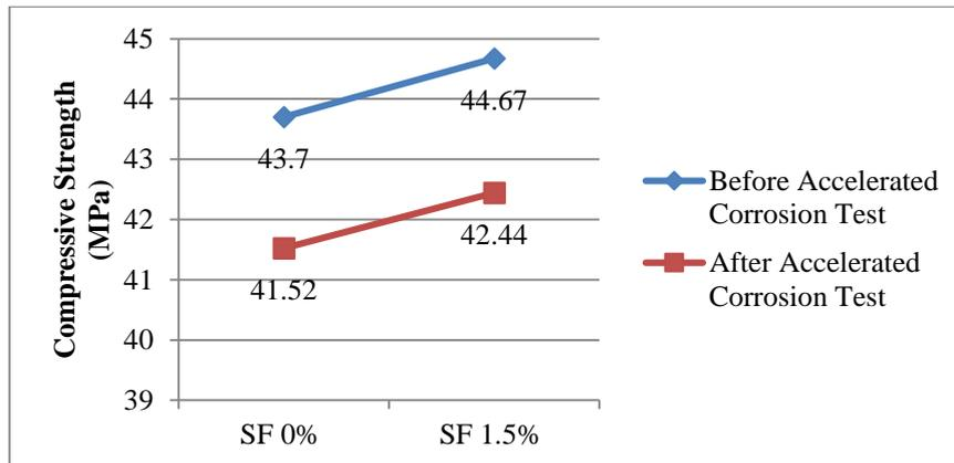
Figure 3: Comparison of compressive strength before and after conducting accelerated corrosion test [12]
