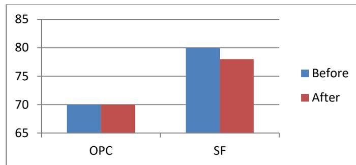
**Figure 4: Comparison of compressive strength before and after corrosion test [6]**
