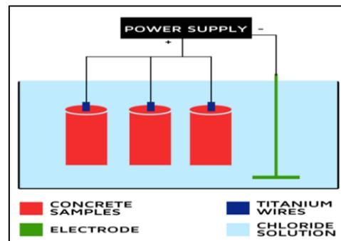
Figure 1: Setup for Impressed Current [6]
