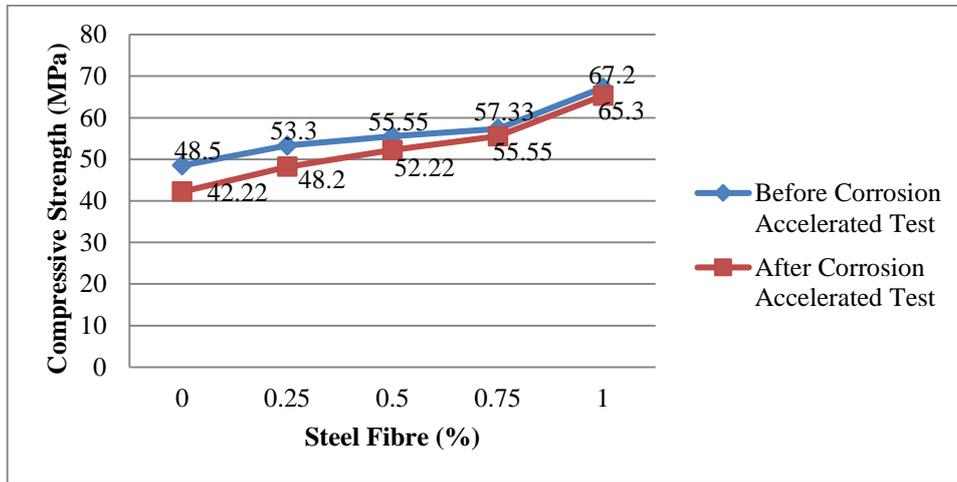
Figure 2: Comparison of compressive strength before and after conducting accelerated corrosion test [16]
