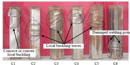
Figure 3.2: Failure Mod for column specimen research Yang and Xu [4].
