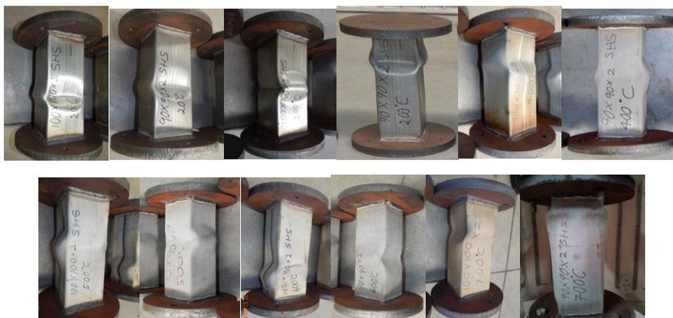
Figure 3.3: Failure Mod for stub column specimen from research Balarupan [5].
