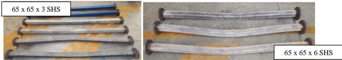
**Figure 3.4: Failure Mod for slender column specimen from research Balarupan [5].**
