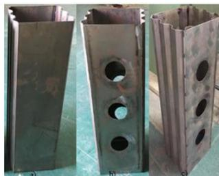
Figure 2.2: a) Column Type 1, b) Column Type 2, c) Column Type 3
