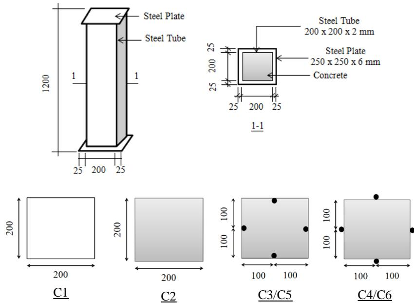
Figure 2.1: Details dimension in research by Yang and Xu [4]
