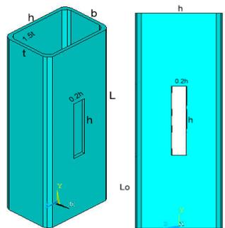
**Figure 2.3: Geometry specimen column in research AL-Shareef [7]**
