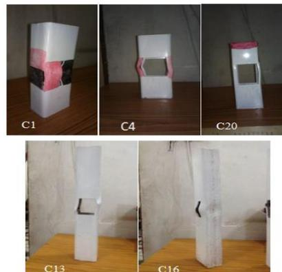
**Figure 3.9:** The picture shows a local buckling on a perforated RHS cross section
