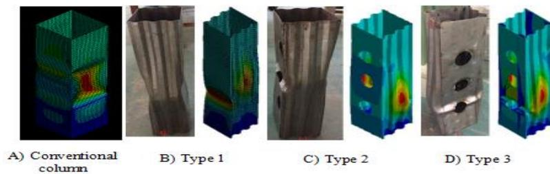
**Figure 3.5: Failure Mod for column specimen from research Varghese and Krishnakumar [6]**
