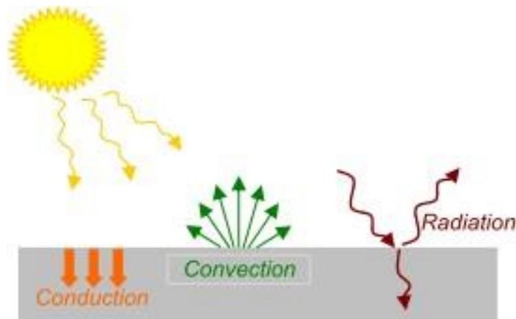
**Figure 2: Heat transfer process in pavement layer [7]**
