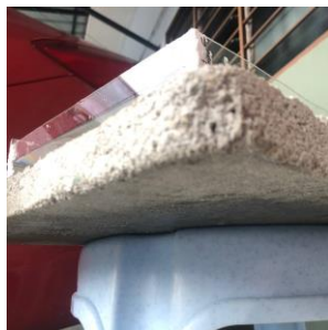
Fig. 14 Seeping water at underside of sample
