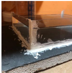
Fig. 16 Permeability test for coating roof
