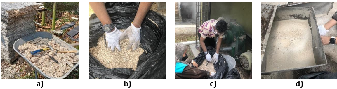
Fig. 1 The process of CWWP preparation a) Cut CWWP; b) Crushed CWWP; c) Process of CWWP grinding; d) Finest particles of CWWP
