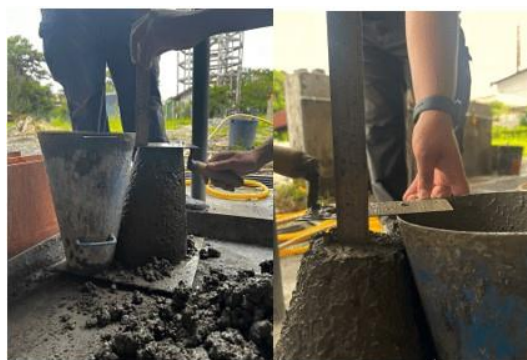
Fig. 7 Slump test for 30% of spent garnet at Advanced Material Laboratory UTHM
