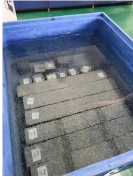
Fig. 8 Curing tank at Advanced Materials Engineering Laboratory UTHM
