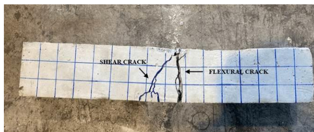
Fig. 18 Final crack patterns with 30% spent garnet replacing sand
