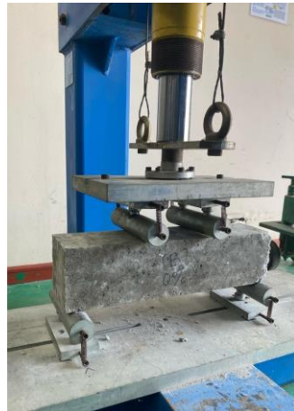
Fig. 4 Bending test in accordance with BS EN 12390: Part 5
