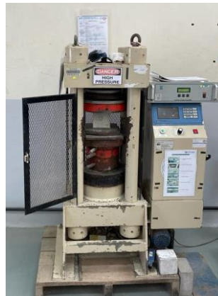
Fig. 3 Compression test in accordance with BS EN 12390: Part 3
