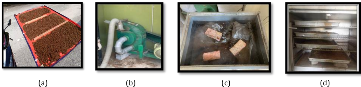
Fig. 2 Preparation of samples (a) Sundry Process, (b) Shredding Process, (c) Hot Water Treatment Process, (d) Oven dry Process
