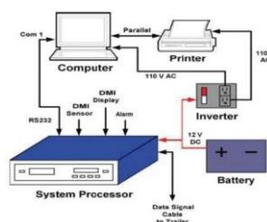
Figure 1: Major component of FWD which control system. [4]
