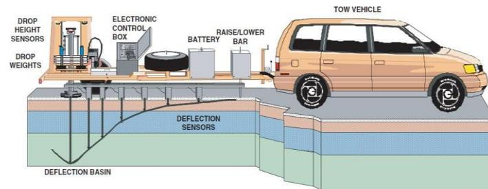
**Figure 3: Type of FWD used in study. [4]**
