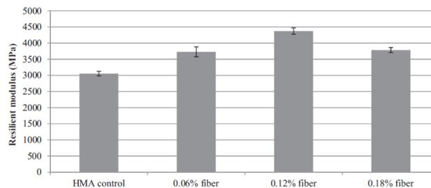
**Figure 4: The resilient modulus test results of asphalt mixtures containing different percentages of polyolefin-glass fiber. [8]**
