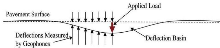
**Figure 2: Schematic drawing of deflection basin measured by geophones. [4]**
