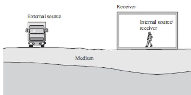
**Figure 1: Example of vibration transmission [5]**
