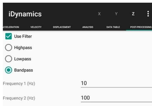
**Figure 6: Band-pass filter option in iDynamics**
