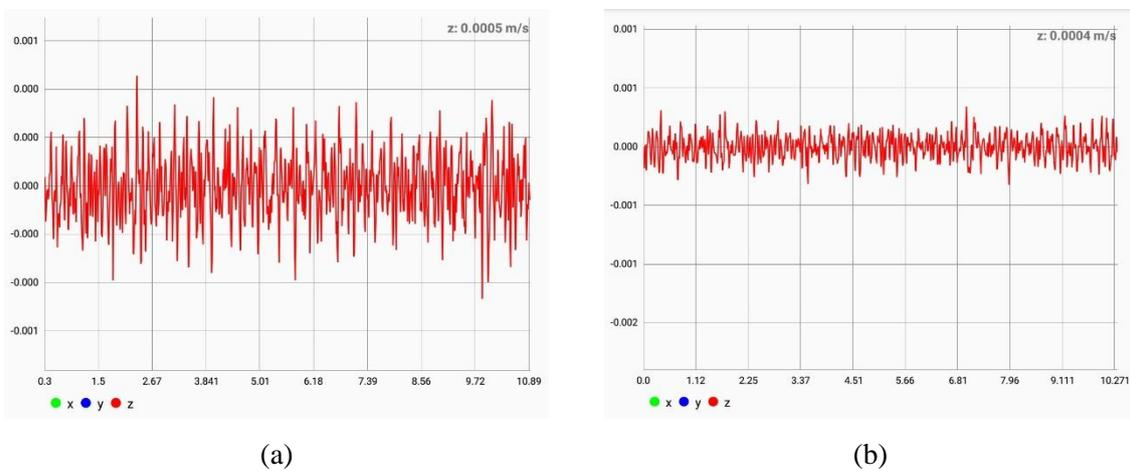
**Figure 7: Vibration velocity on 28<sup>th</sup> November 2020 at 2pm (a) 2 m (b) 8 m**
