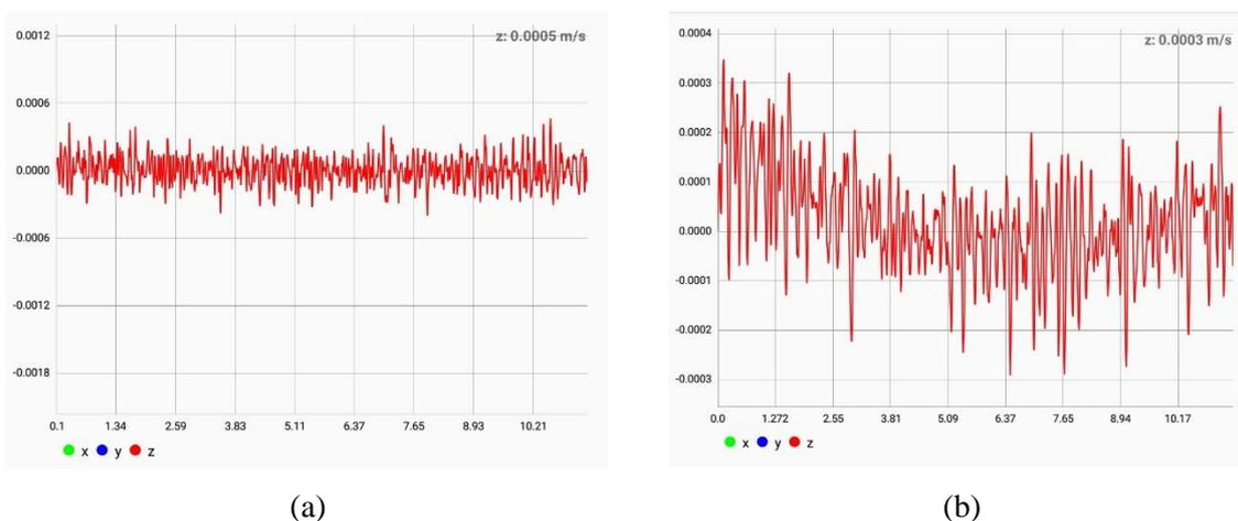
**Figure 8: Vibration velocity on 29<sup>th</sup> November 2020 at 9 am (a) 2 m (b) 8 m**
