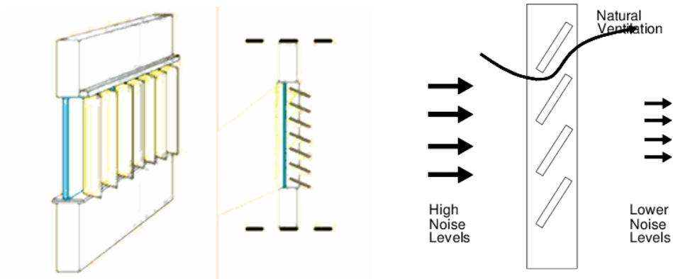
**Figure 7: Louvres allowing natural air flow while reducing the noise impact**
