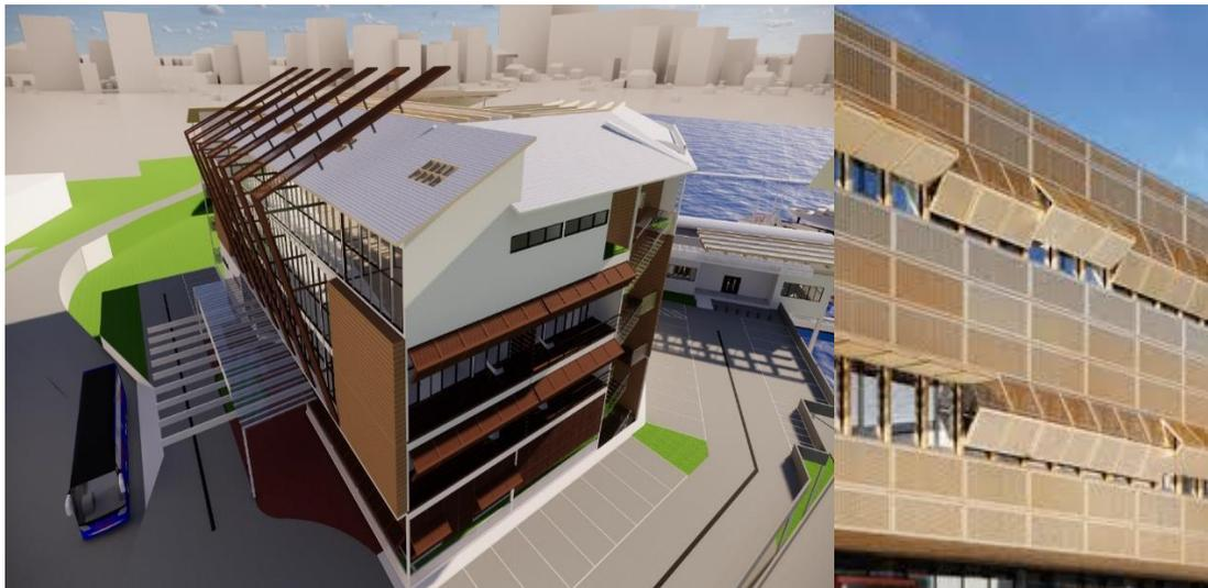
**Figure 6: ‘HOP (B) : NOB’ Marina Quay proposed design showing the side to be applied with the Adjustable Folding Aluminium Louvres**
