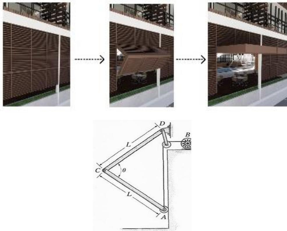
**Figure 8: The Working Mechanism of Adjustable Folding Aluminium Louvres**
