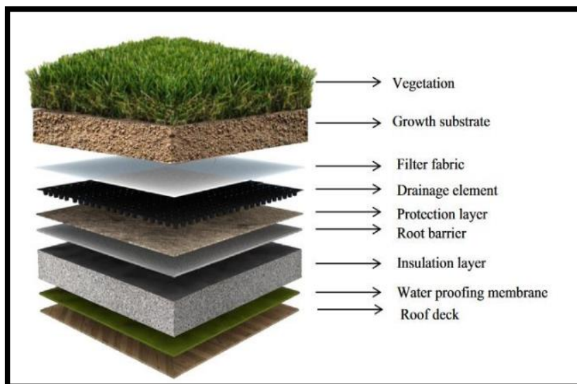
Figure 4: Cross Section of a Green Roof [9]
