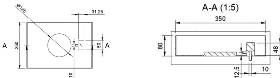
Figure 3: Cross sectional (left) and Top (right) View of Buoyancy Control Device
