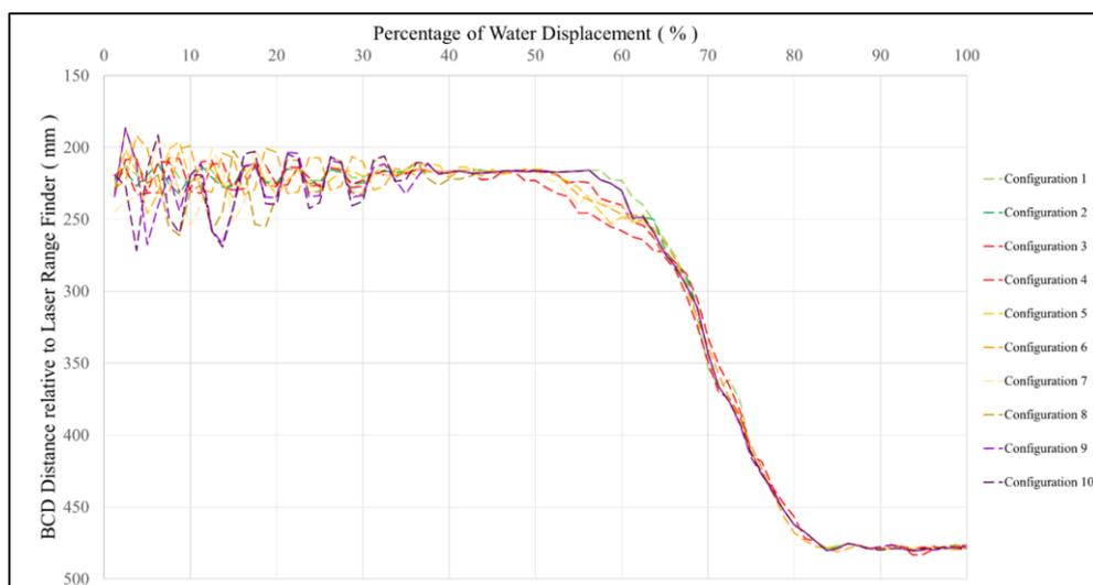
**Figure 8: Graph of BCD Distance Relative to Laser Range Finder Against Percentage of Water Displacement**
