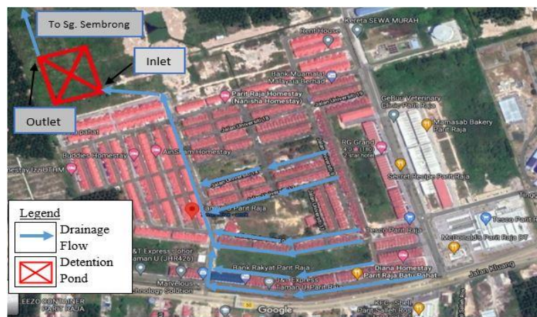
Figure 13: Proposed location for the dry detention pond at Taman Universiti, Parit Raja
