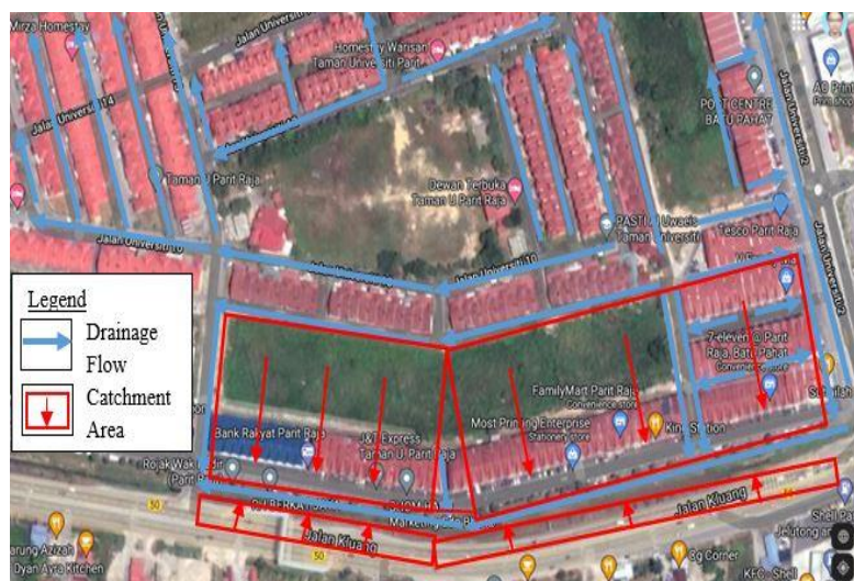
Figure 9: Drainage flow and surface runoff from catchment area that will flow into the drain
