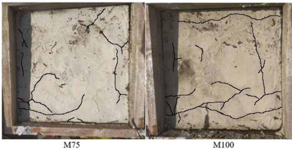
Figure 17: Uncured panel specimens for M75 and M100 at 30 th day
