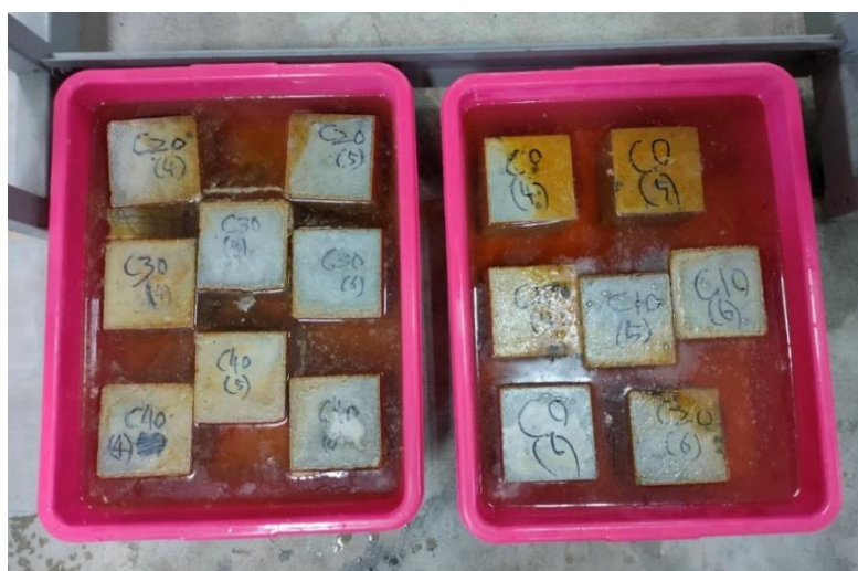
Figure 4 : Immersion of concretes in 5% hydrochloric acid solution for duration of 28 days.
