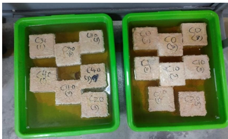
Figure 5: Immersion of concretes in 5% sulphuric acid solution for duration of 28 days.
