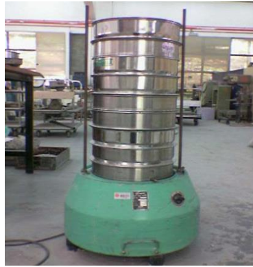
Figure 2: Mechanical Sieve Shaker
