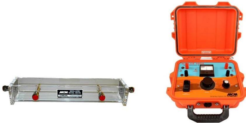
Figure 3: Soil box and M.C. Miller Resistivity Meter, 400A
