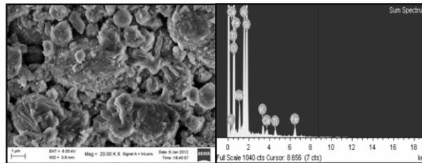
**Figure 1: SEM micrograph of FA geopolymer [7]**
