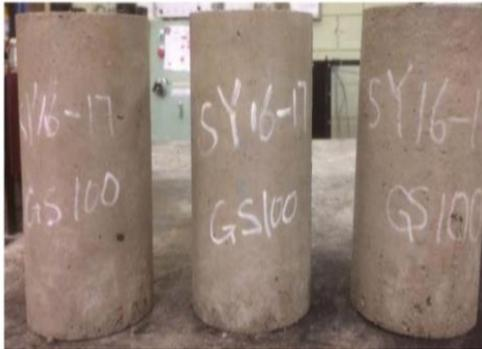
Figure 1: Cylinder concrete specimen
