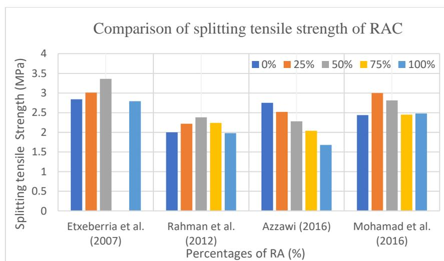
**Figure 6: Splitting tensile strength of RAC**
