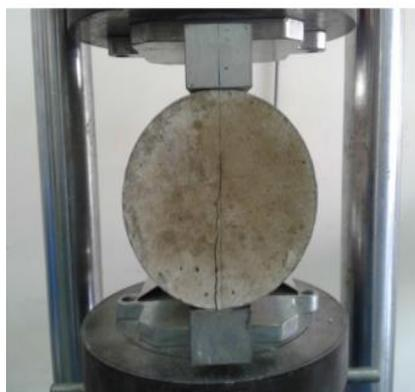
Figure 3: Split tensile strength test
