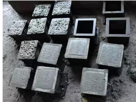
Figure 2: Cube concrete specimen
