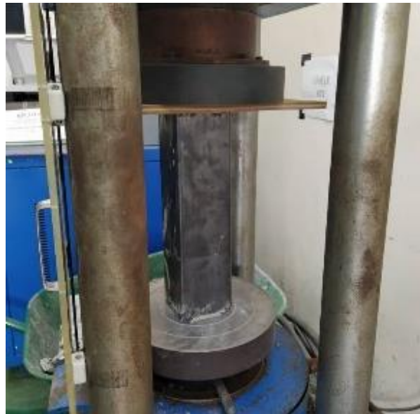
Figure 1: Compression test on modified foam concrete filled hollow section (FCFHS)
