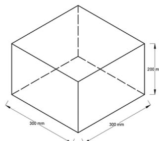
**Figure 1: Dimension of the MRC block**
