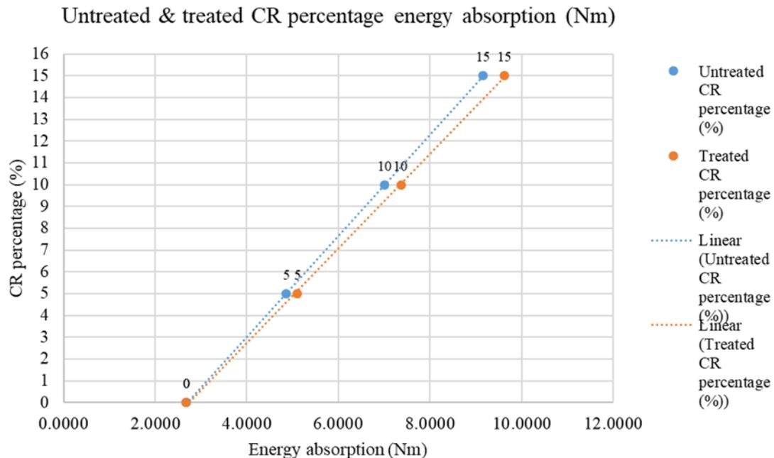
**Figure 4: Untreated & treated CR percentage energy absorption**
