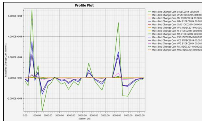
Figure 17: Individual Particle Size Gradation’s Cumulative Bed Volume Change Distribution along Sg. Bertam
