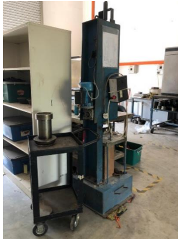
Figure 2: Marshall Compactor Machine
