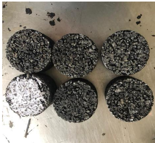
Figure 3: Cold Mix Asphalt specimens
