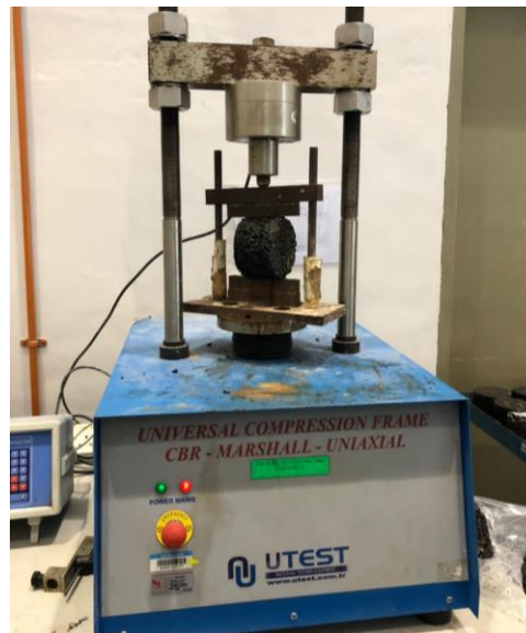
Figure 4: Universal Compression Frame Marshall Test Machine (UTM)
