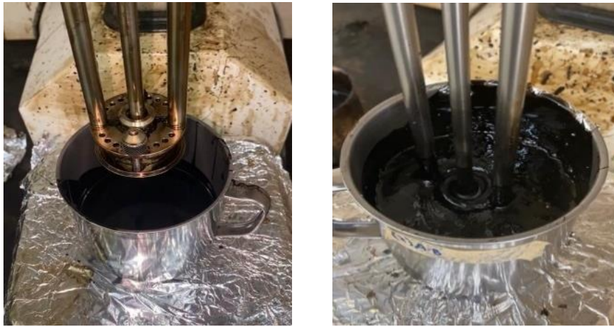
Figure 2: Blending process of asphalt PEN60/70 and SBR coagulum modified binder
