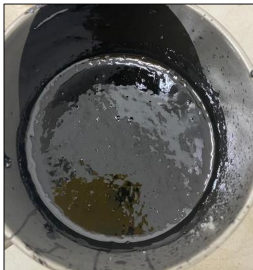
Figure 3: The homogenous blend of SBR modified binder at 2000 rpm
