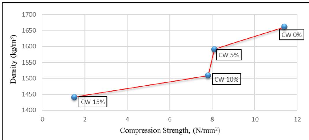
**Figure 6: Relationship between compressive strength and density for 7 days**
