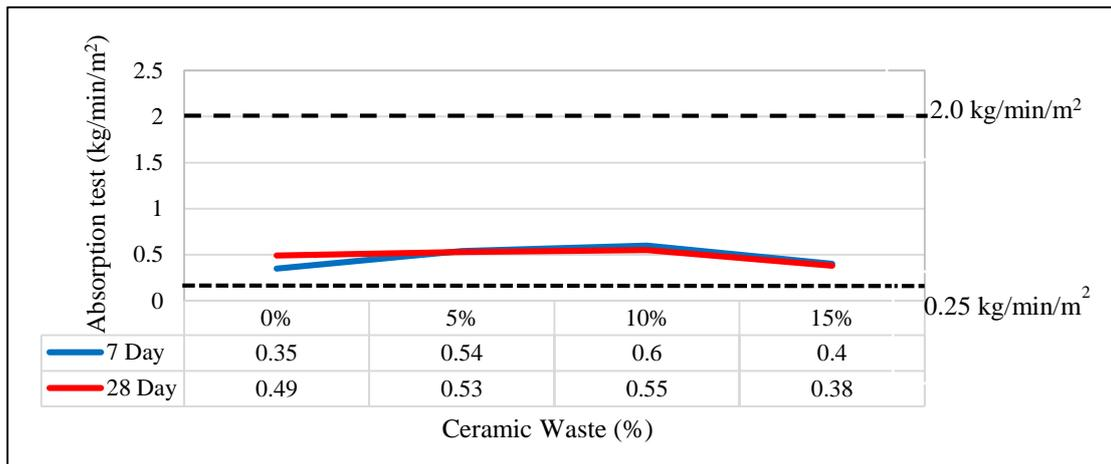
Figure 4: The initial absorption rate of the brick sample is proportional to the percentage of ceramic waste
