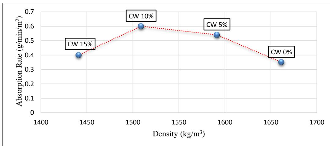
**Figure 8: Relationship between the density and absorption rate for 7 days**
