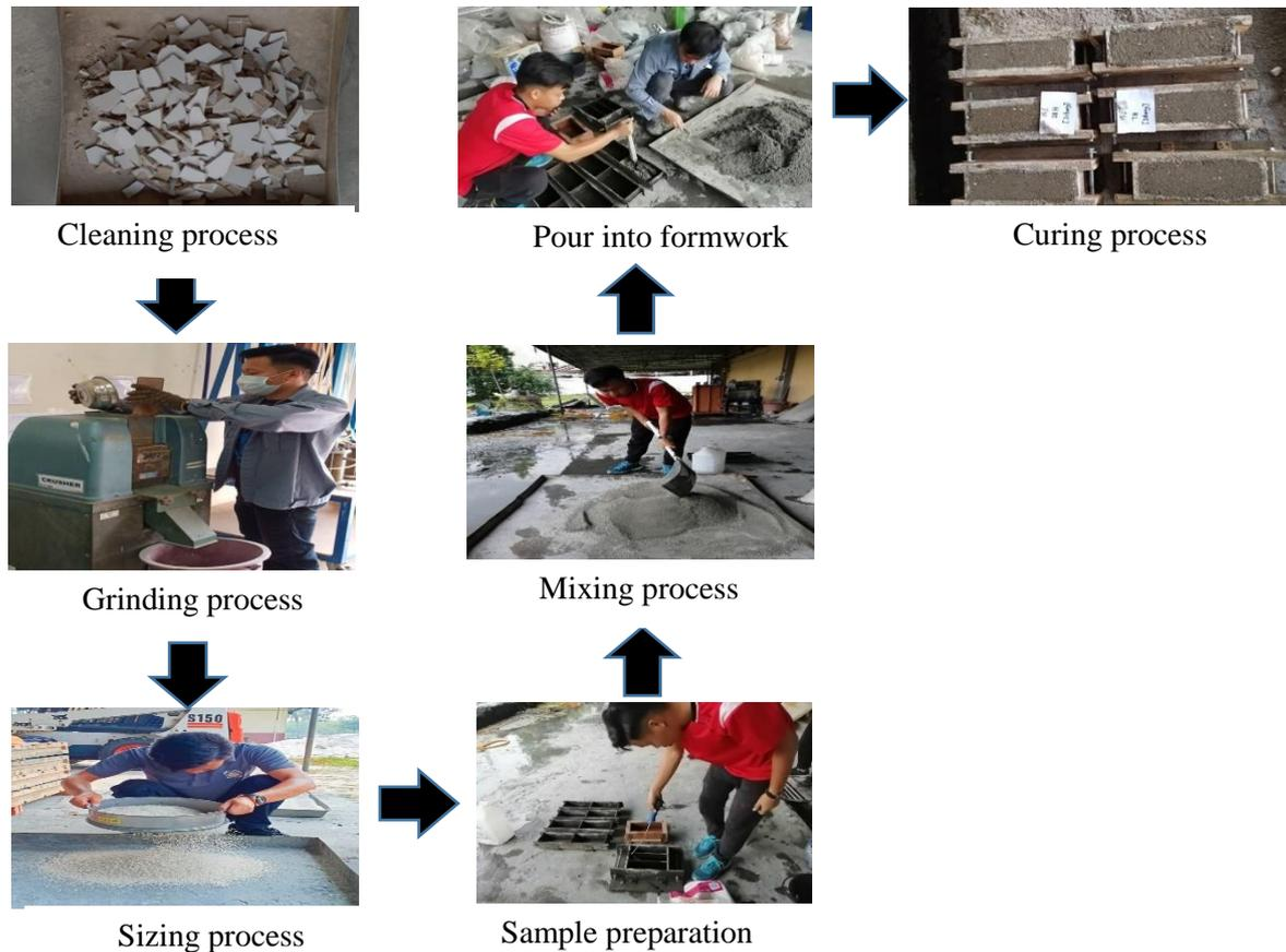
**Figure 1 : Flow chart of fabricating process of CWB**
