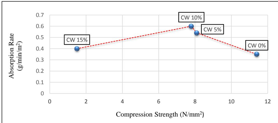
**Figure 10: Relationship between compressive strength and absorption for 7 days**
