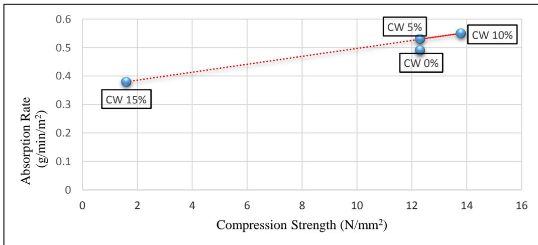
**Figure 11: Relationship between compressive strength and absorption for 28 days**
