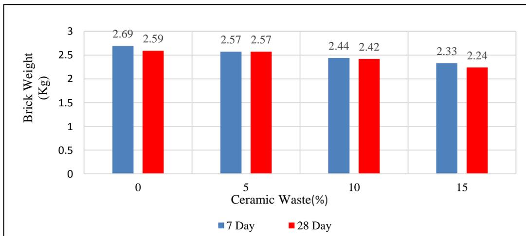
**Figure 2: Relationship between brick sample weight to ceramic waste percentage**
