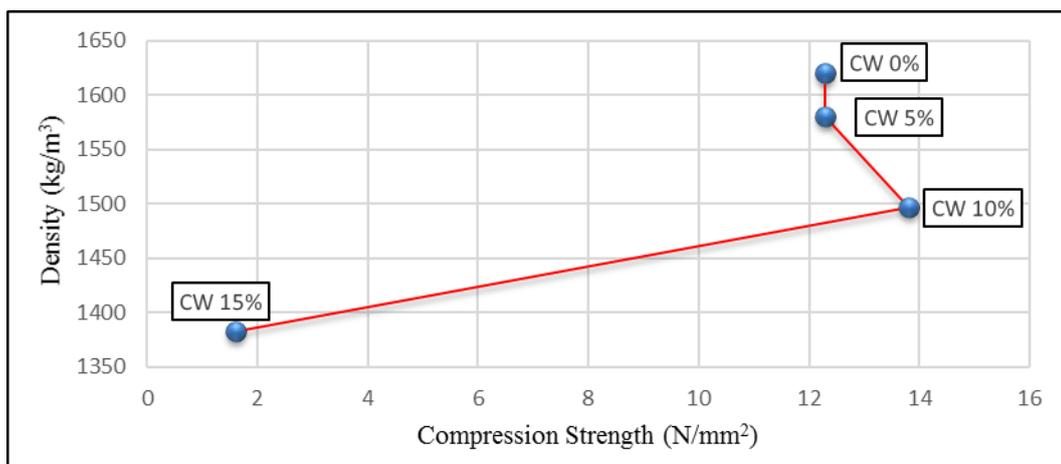
**Figure 7: Relationship between compressive strength and density for 28 days**
