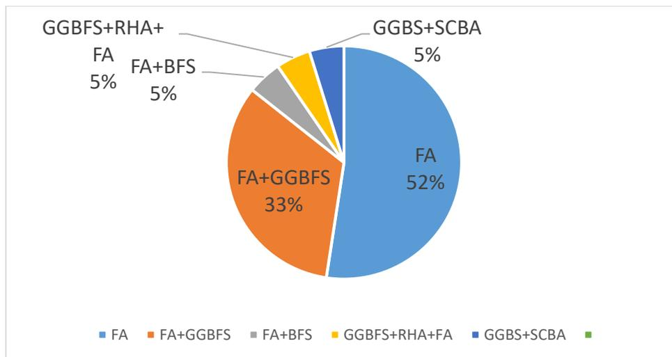
**Figure 2: Materials mixtures of geopolymer concrete**
