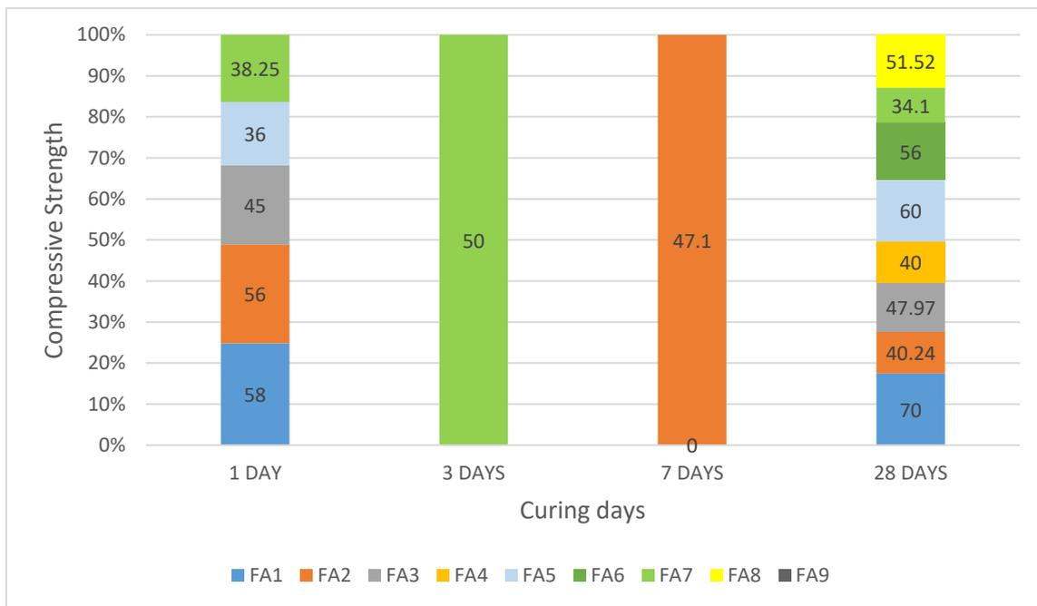
**Figure 4: The effect of curing days on compressive strength of geopolymer concrete**
