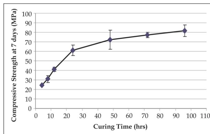
**Figure 3: The effect of curing days on compressive strength of geopolymer concrete**
