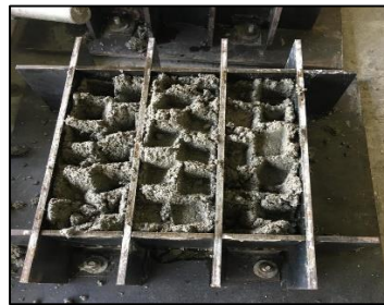
Figure 3: Compaction of brick.
