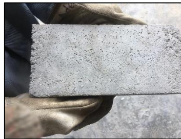
Figure 9: The condition of the brick after drop.
