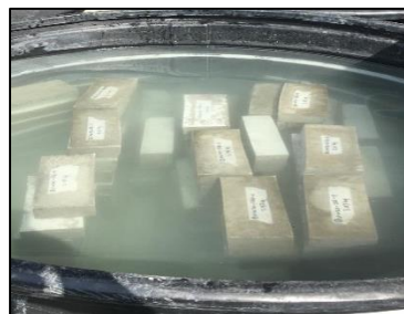
Figure 4: Water curing of brick sample.
