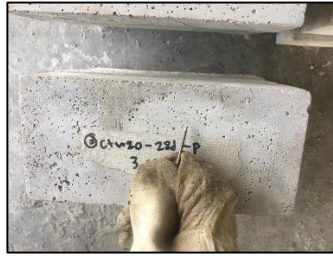
Figure 8: The surface condition of the brick after the scratch.
