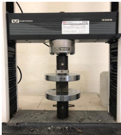
Figure 2: Compressive strength test
