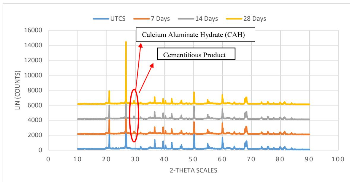
**Figure 1: The XRD Results for (3%L+9%P) Stabilizer Proportion**
