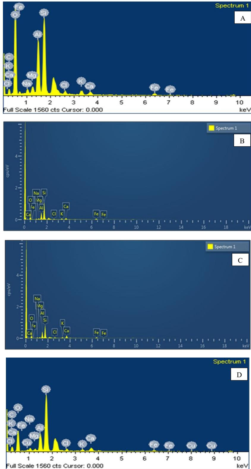
Figure 3: EDX Results for Untreated (A) and (3%L+9%P) at different curing times, 7 days (B), 14 days (C) and 28 days (D)
