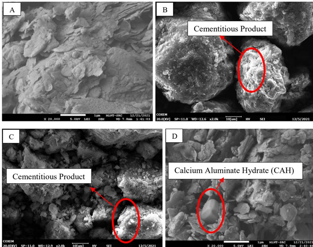
**Figure 2: The SEM Image for Untreated Sample (A) and (3%L+9%P) at different curing times, 7 days (B), 14 days (C) and 28 days (D)**
