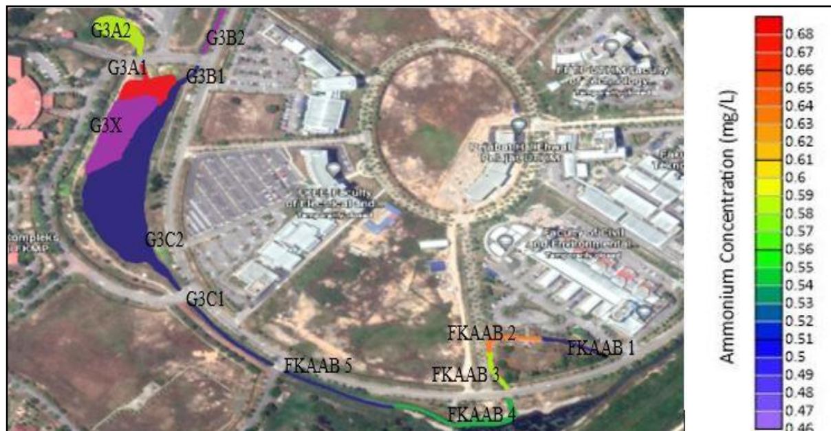
Figure 4: Ammonium concentration map along the Faculty of Civil Engineering and Built Environment and G3 Lake in week 2
