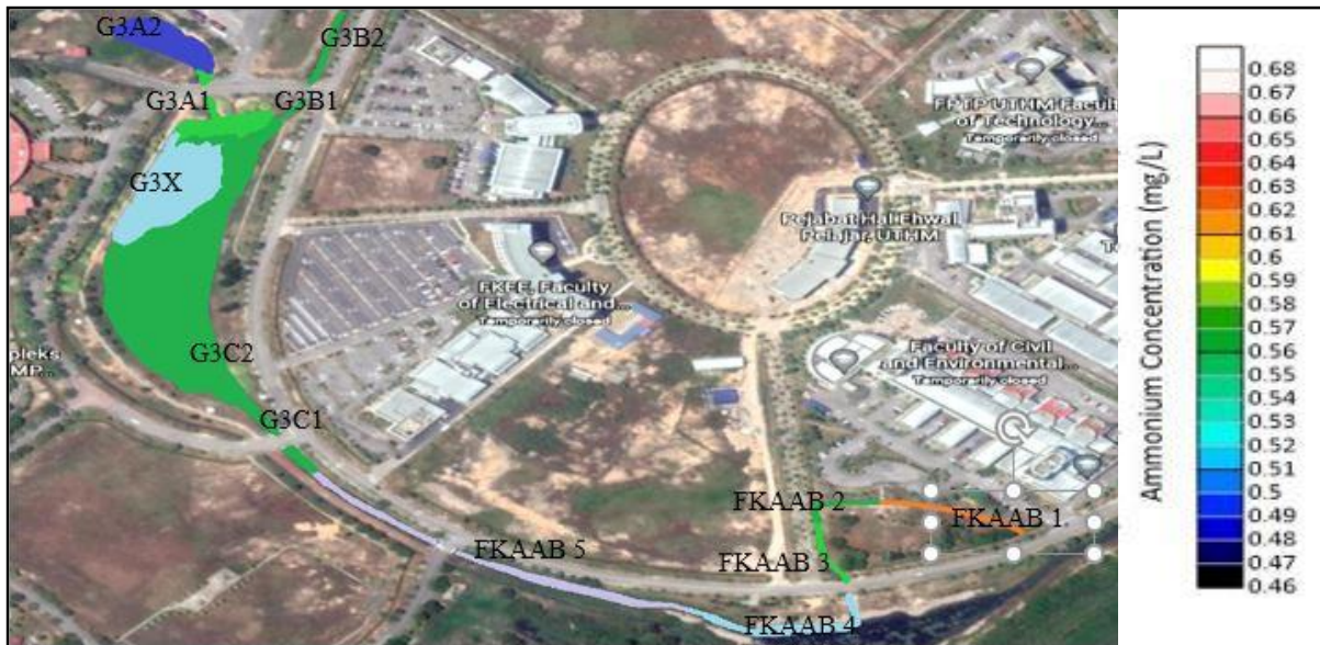
Figure 5: Ammonium concentration map along the Faculty of Civil Engineering and Built Environment and G3 Lake in week 3
