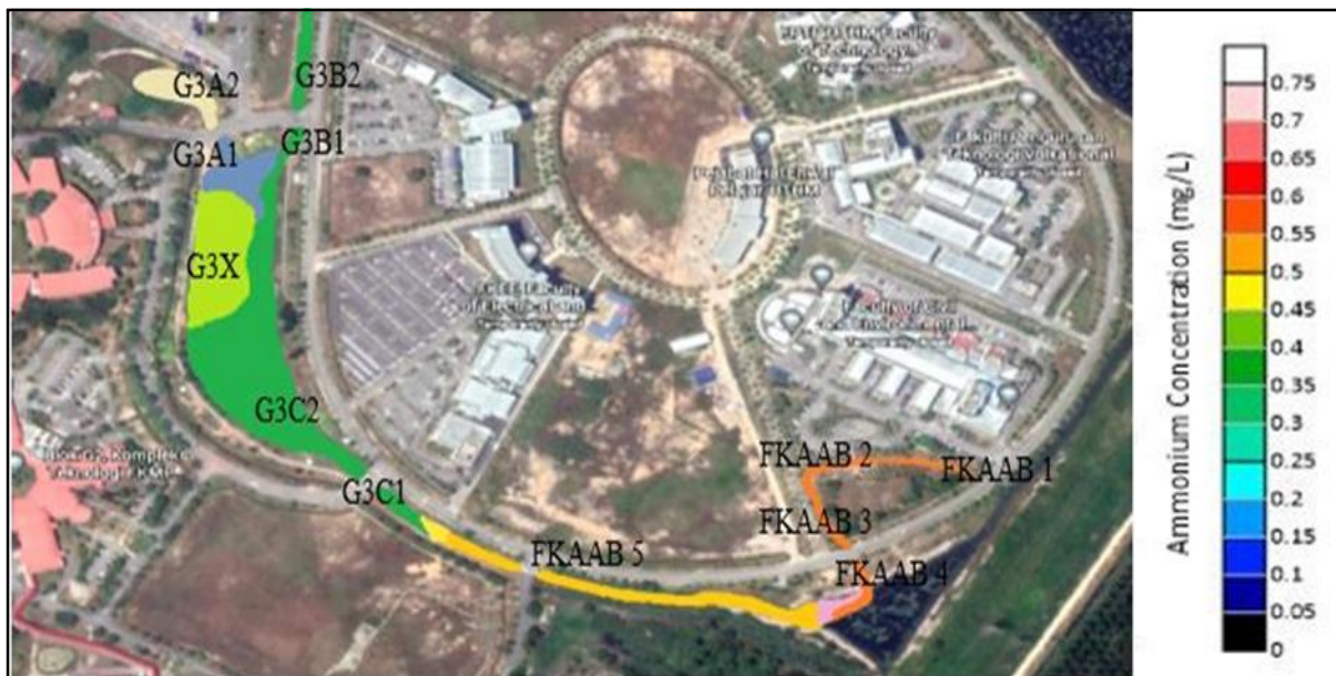
Figure 3: Ammonium concentration map along the Faculty of Civil Engineering and Built Environment and G3 Lake in week 1
