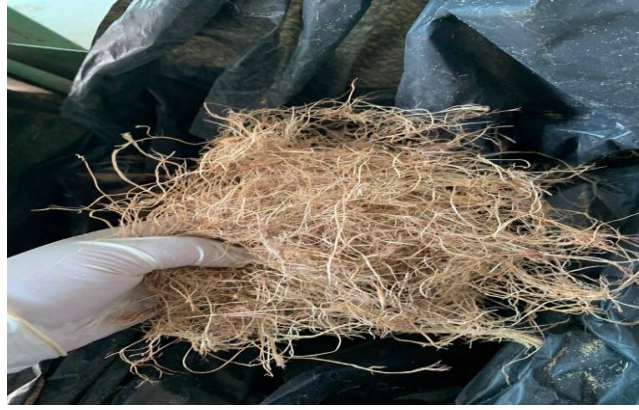
Figure 1: EFB Fibres after shredding process
